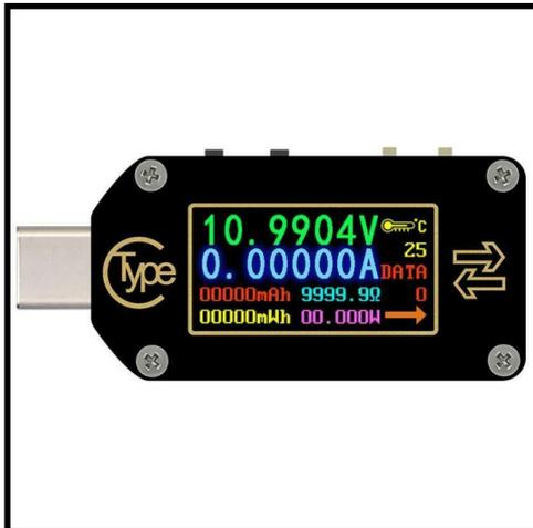
The TC66C is a small but multifunctional USB C multimeter. Due to the support of current Quick Charge Standards it can also be used in conjunction with current handheld hardware.
