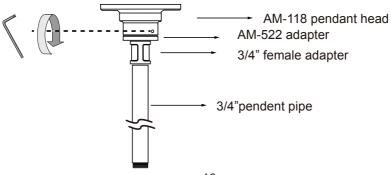
3. Route Ethernet cable and other wires through the pendant head. You may apply a 1 inch conduit.
