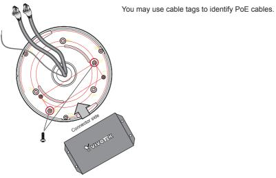
4. In a cascade topology, there should be 2 Ethernet cables in the pipe. One is used as PoE input, the other as the out port to the next conduit box.
