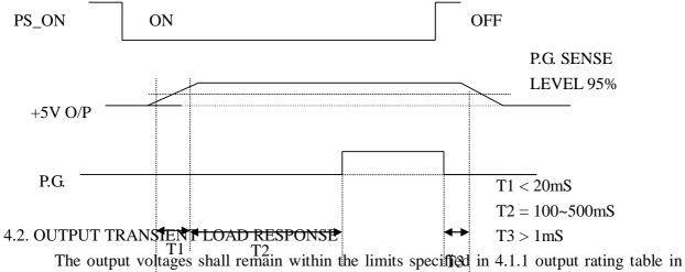
The output voltages shall remain within the limits specified in 4.1.1 output rating table in page 4 for the step loading and within the limits specified in Table 1 for the capacitive loading. The load transient repetition rate shall be tested between 50Hz and 5 kHz at duty cycles ranging from 10%-90%. The load transient repetition rate is only a test specification. The step load may occur anywhere within the MIN load to the MAX load shown in Table 1.
