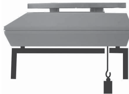
Fig. 1: Setup of balance for underfloor weighing
