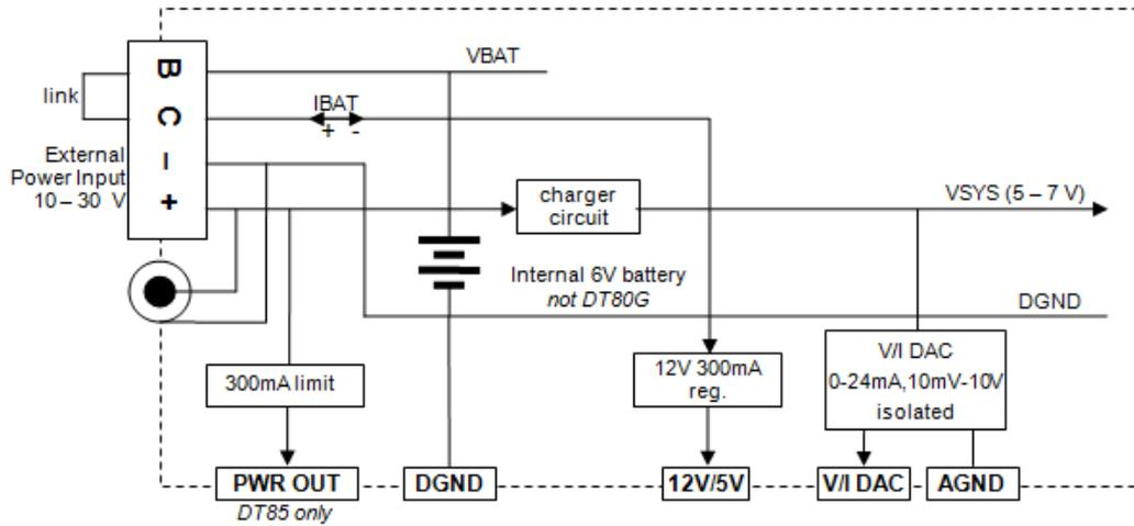
Figure 120: DT80/ 82I/ 85 series 4 internal power subsystem
