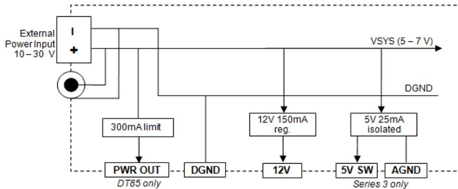
Figure 121: DT82E/ 80L/ 85L series 2 and 3 internal power subsystem
