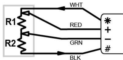
Figure 152: Wiring for 4-wire Carlson Sensor
