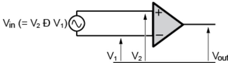
Figure 179: Common-mode voltage  $V_{CM}$  and Differential voltage ( $V_{Diff}$ ) — 2
