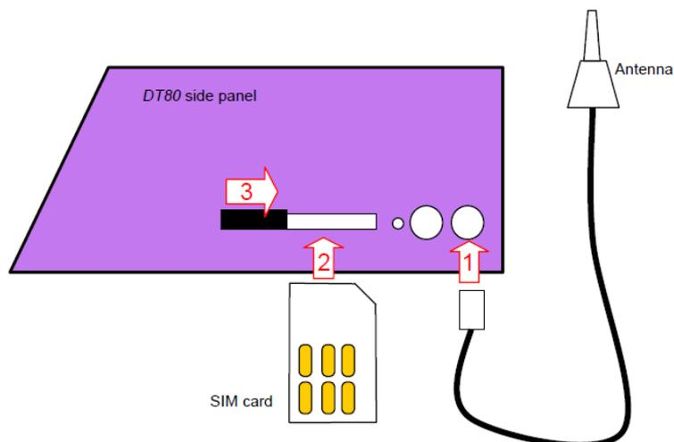
Figure 82: Connecting the antenna and SIM card
