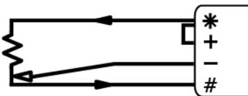
Figure 133: Wiring for 3-wire resistance input
