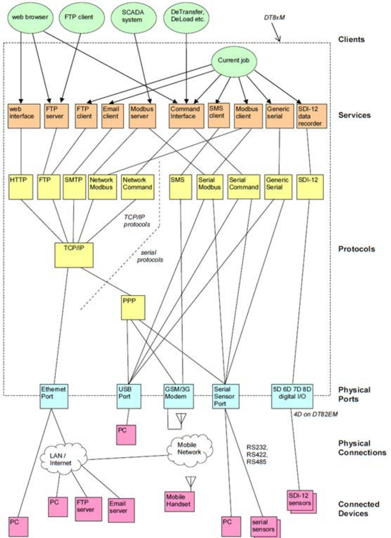
Figure 72: DT80 communications options (integrated modem models)
