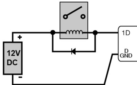
Figure 157: Wiring for driving an external relay
