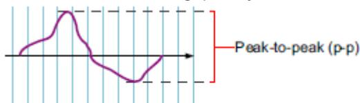
Figure 180: Peak-to-peak measurement
