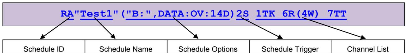
Figure 7: Components of a typical schedule command
