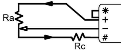
Figure 144: Wiring for 3 wire bridge input using internal current excitation
