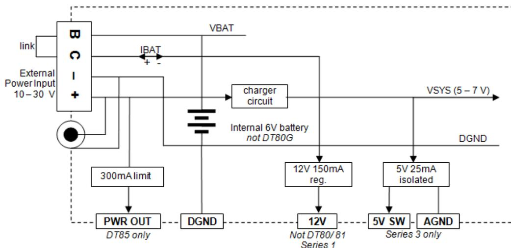
Figure 119: *DT80/82/85* series 2 and 3 internal power subsystem
