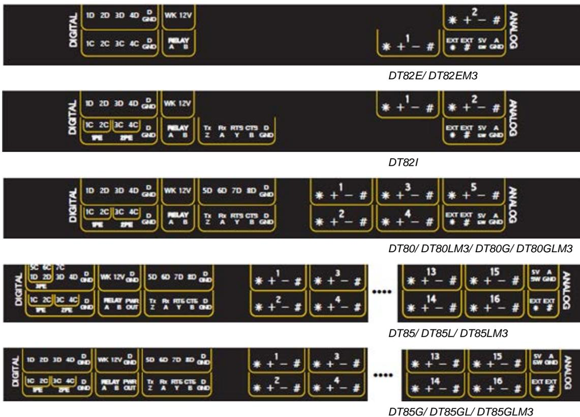
Figure 110: Standard terminal labels for DT80, DT82 and DT85 on Series 3
