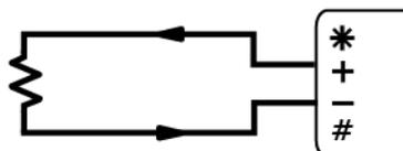
Figure 136: Wiring for 2-wire independent resistance input (Series 3 and 4)
