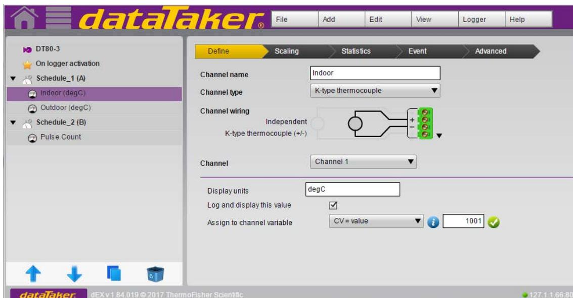
Figure 23: Typical configuration builder display
