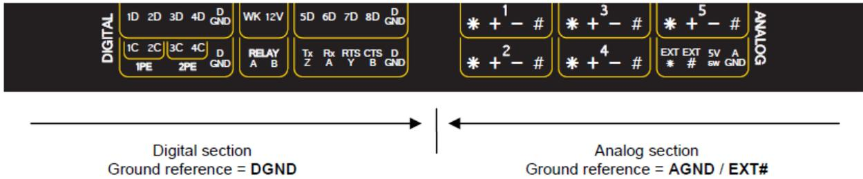
Figure 170: The DT80 has two ground systems
