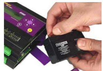
Figure 115: How to remove the main battery
