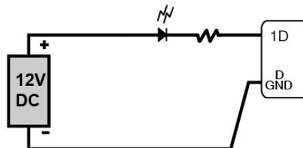
Figure 158: Wiring for driving an external LED
