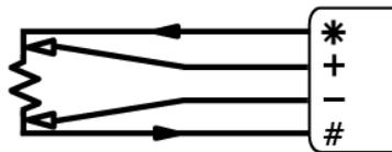
Figure 132: Wiring for 4-wire resistance input
