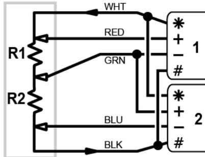
Figure 151: Wiring for 5-wire Carlson Sensor
