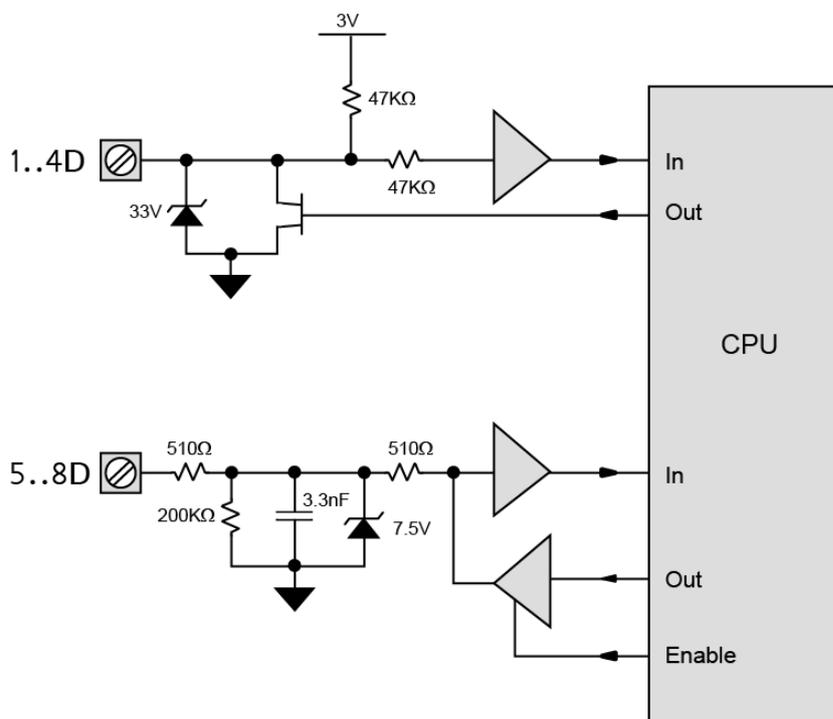
Figure 154: Digital Circuit (DT80 channel numbers shown)
