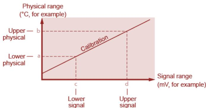
Figure 17: Span coordinates
