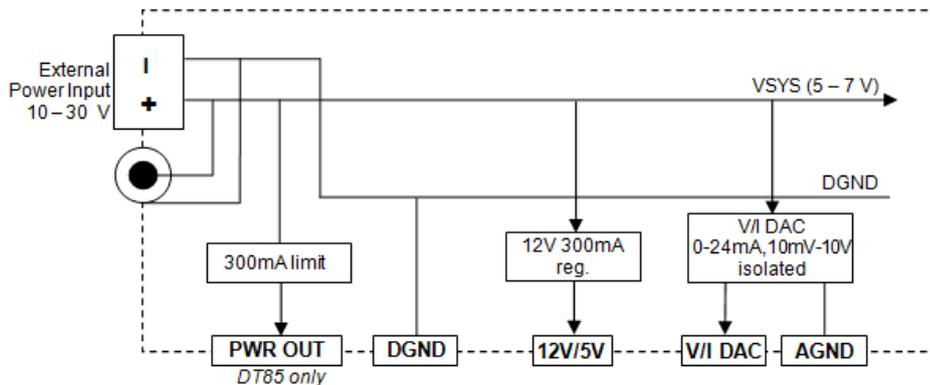
Figure 122: DT82E/ 80L/ 85L series 4 internal power subsystem
