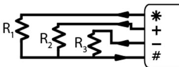
Figure 137: Wiring for 2-wire shared terminal resistance inputs (Series 3 and 4)
