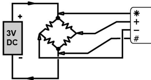
Figure 140: Wiring for 6-wire bridge using external voltage excitation
