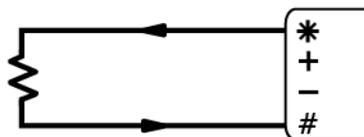
Figure 135: Wiring for 2-wire independent resistance input
