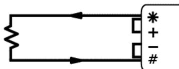
Figure 134: Wiring for 2-wire resistance input
