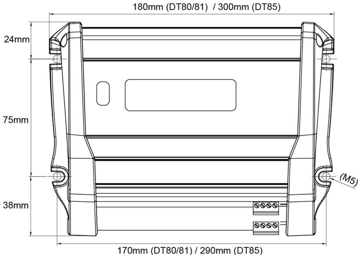
Figure 117: Mounting hole positions and overall dimensions
