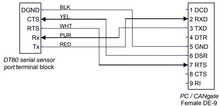
Figure 177: Serial Sensor RS-232 Null Modem Cable (CAB-015)
