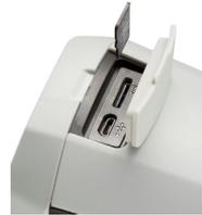
→ **If the memory card is not recognised when triggering memory with the red trigger button (9) for image storage (card symbol with a red X on the display), check the memory capacity, the correct fit or the correct data formatting (FAT32) of the memory card.**
