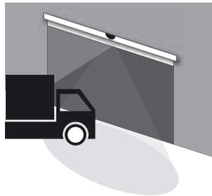
\*) Vehicles crossing the detection range of the sensor may cause the human-presence relay to be activated unexpectedly.
