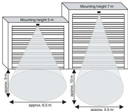
At maximum sensitivity and angle of incidence
