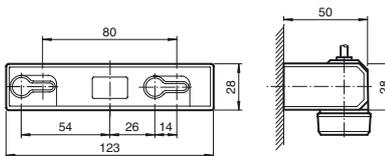
Mounting dimensions with mounting bracket set AIR30
