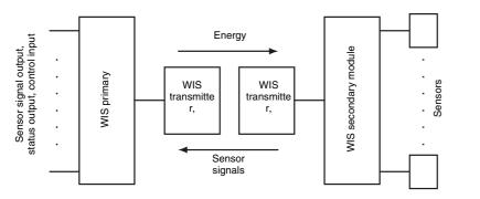
The sum of the currents of all sensors attached to the WIS secondary module must not be greater than the maximum transferable current. This is calculated by dividing the transferable power by the 12 V provided by the transmitters.
