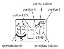
• For optimal setting, now turn the sensitivity adjuster to the middle position between the positions A and B.
