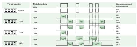
Time  $t_{ON}$ ,  $t_{ON}$  and  $t_{IOFF}$  are adjustable from 0.1 to 10 seconds. The H/D Switch (Left, outer switch) is shown in the "Dark ON" position.
