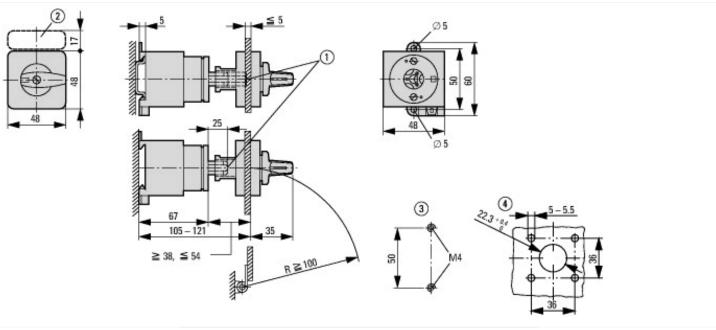
(1) Shaft extension with ZAV-T0 possible, max. 4 x 25 = 100 mm (2) ZFS-... Label mount not included as standard
