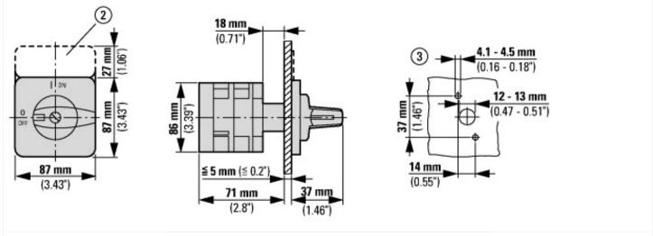
② ZFS-... Label mount not included as standard ③ Drilling dimensions door Cam switches T5B and T5 are of identical design, only their contacts are different
