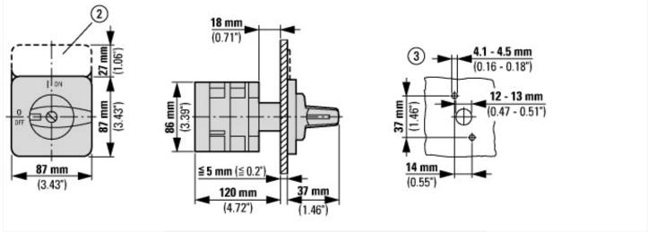
② ZFS-... Label mount not included as standard ③ Drilling dimensions door Cam switches T5B and T5 are of identical design, only their contacts are different
