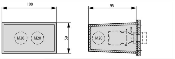
Cable gland: 4 x M20 Construction type: one-piece
