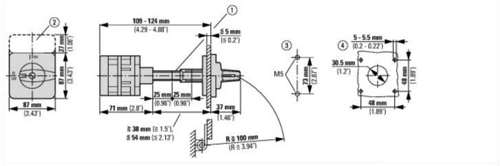
Shaft extension with ZAV-P3 possible, max. 4 x 25 = 100 mm
