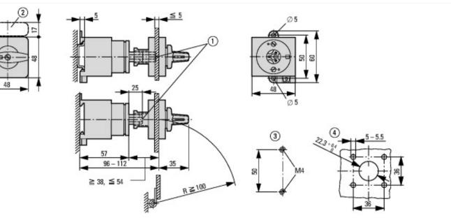
① Shaft extension with ZAV-T0 possible, max. 4 x 25 = 100 mm
