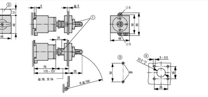
(1) Shaft extension with ZAV-T0 possible, max. 4 x 25 = 100 mm
