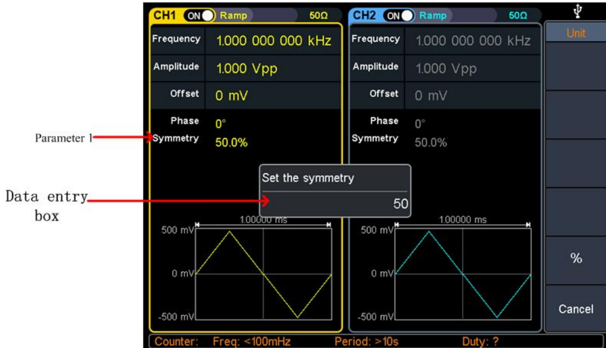
Figure 4- 5: Set the symmetry of ramp wave
