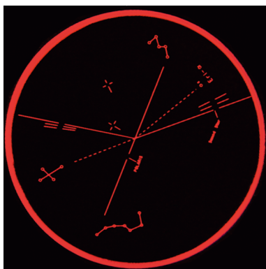
Illustration 6: Polar finder scope engraving plate with Big Dipper (bottom) and rotated RA axis.
