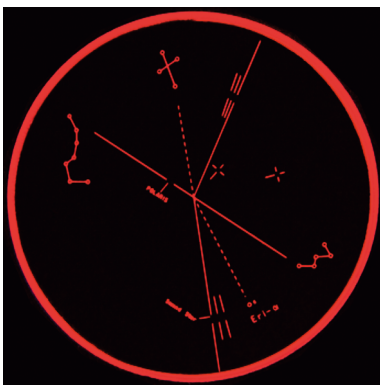
Illustration 4: Polar finder scope engraving plate with Big Dipper (left).
