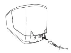
2 Plug the AC Power Cord into an AC power outlet.
