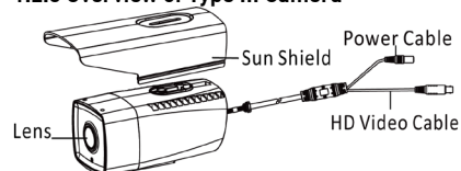
Figure 1-2 Overview of Type II Camera
