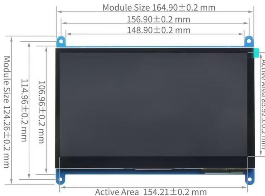
Screw hole diameter: 3 mm.
