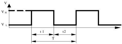
$$T = \frac{1}{f_{\text{PWM}}} = t1 + t2 (\text{sec}) \quad .$$
