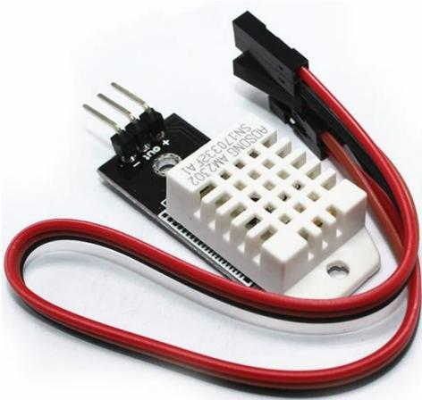
This sensor measures the humidity and temperature of the surrounding air with its capacitive humidity probe and thermistor and displays a digital signal output. Therefore, analog pins are no longer necessary.
