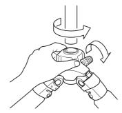
3. Remove the upper part of center column. Loosen the center column stopper and the center column stopper. Pull out the upper part of center column from the main body.
