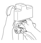
When attaching the camera to the pan head, check to make sure that the quick release shoe is engaged in the catch of the pan head before locking the lever.
