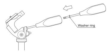
Remove the vertical tilt handle from the pan head, and screw into the back of the pan & tilt handle.
