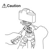
When loosening either the pan & tilt handle, or the vertical tilt handle, take precaution by keeping a firm grip on the handle until the pan head is locked down.
