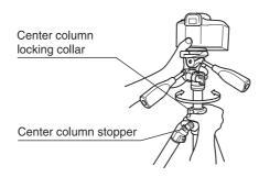
Hold onto the pan head with one hand, and loosen the center column locking collar with the other hand. Raise or lower pan head to desired height, and while maintaining a hold of the pan head, tighten the locking collar.
