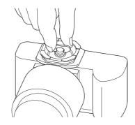
Align the length of the quick release shoe along the base of the camera body, and securely tighten the mounting wing nut.
