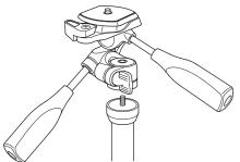
1. Remove the pan head when inverting &/or replacing the center column.
