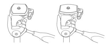
The quick release shoe can be attached to the camera body in either directions (along the length, or along the width).
