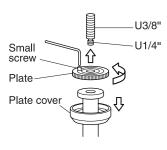
The pan head fixing screw is reversible for either large thread (U3/8") or small thread (U1/4").
