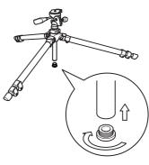
Screw in the center column base stopper to the bottom of the upper part of center column.
