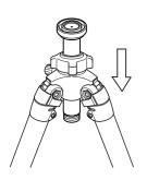
4. Pull in the lower part of center column from the top of the main body.
