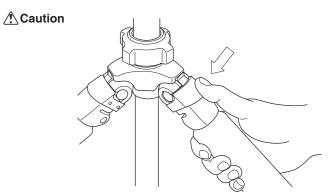
After choosing the desired leg angle, securely push in the adjustment lock.
