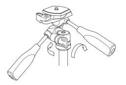
Set the new head, or accessory on the tripod's threaded post, and turn clockwise until it comes to a stop.
