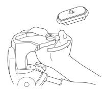
To remove the quick release shoe from the pan head, turn quick release lock lever and lift out quick release shoe from its back.
