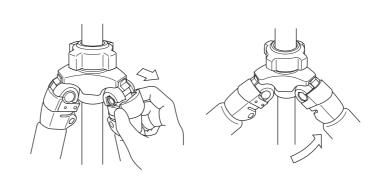
To change the angle of each leg, close the leg slightly and then pull the leg angle adjustment lock out. There is a choice of two other angle positions.
