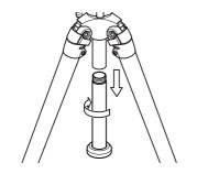
2. Remove the lower part of center column. Hold the upper part of center column and turn the lower part of center column.
