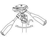
Loosen the panning lock knob, and the head will rotate along the horizontal direction.
