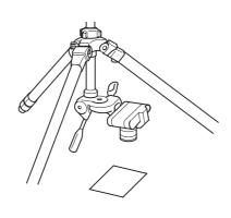
6. By inverting the center column, it is possible to do copy, and close up work.
