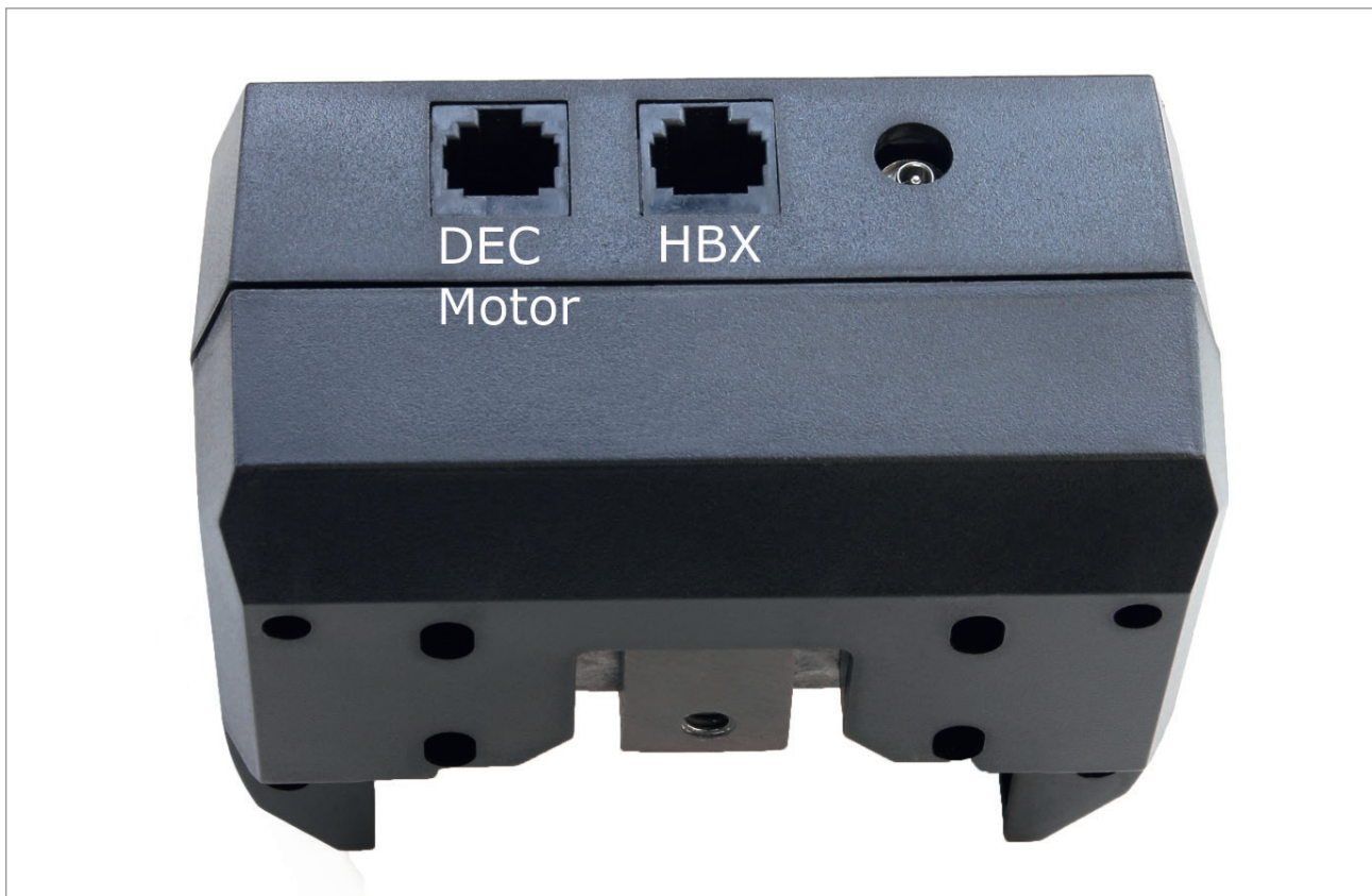
Fig. 1c: Control-Panel of DEC Motor
