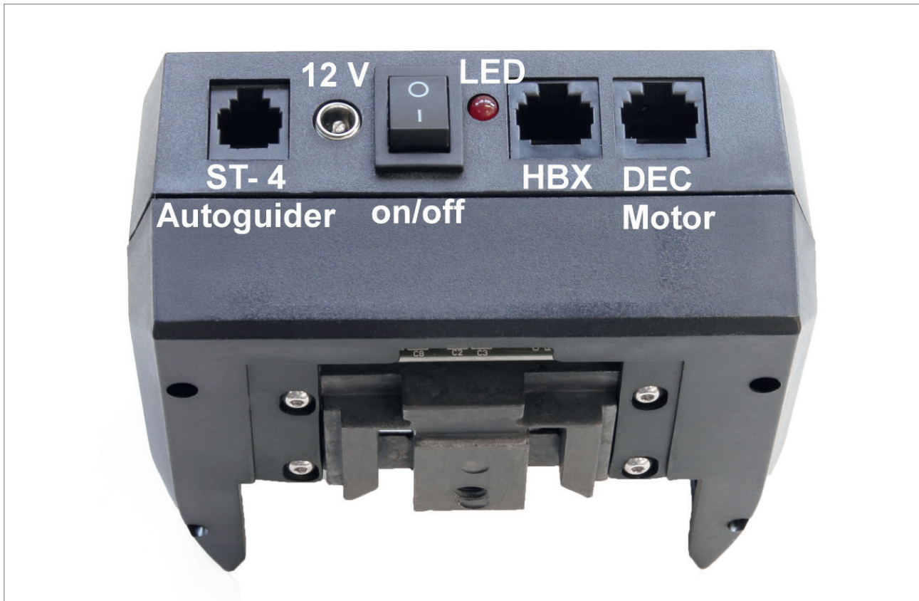
Fig. 1b: Control-Panel of RA motor
