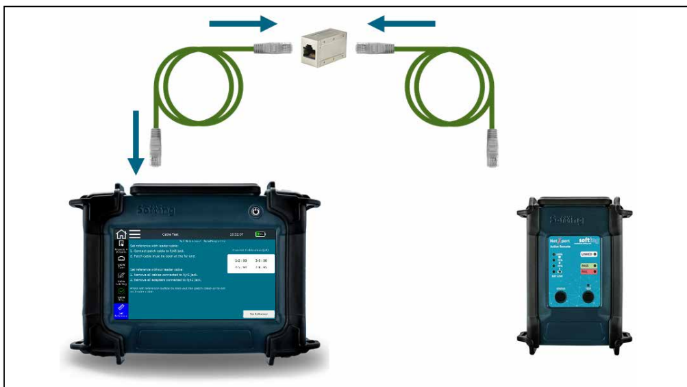
Figure 25 – Test setup for setting the reference
