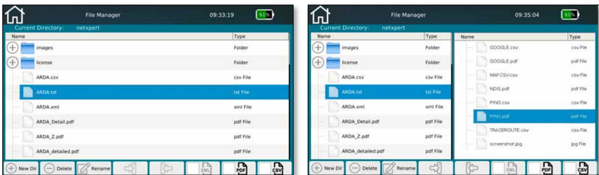
Figure 40 – File Manager (left only internal memory, right internal and external memory with connected USB drive)
