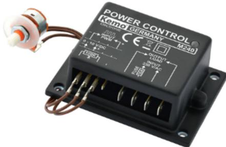
Power controller for 230 V/AC consumers such as motors, lamps, many dimmable LEDs etc. The controller is overload- proof and can be controlled via a potentiometer (100 K lin.), a control voltage (0 - 10 V) or with PWM signals (0 - 100%, 100 - 10,000 Hz).
