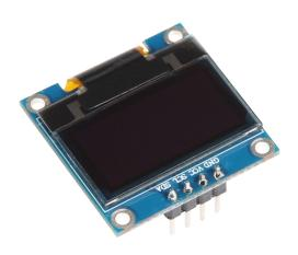
This small but nice display with a black background and blue display figure color is controlled with I<sup>2</sup>C which enables multiple applications. The high resolution offers a sharp picture which meets highest requirements with the lowest space requirement.
