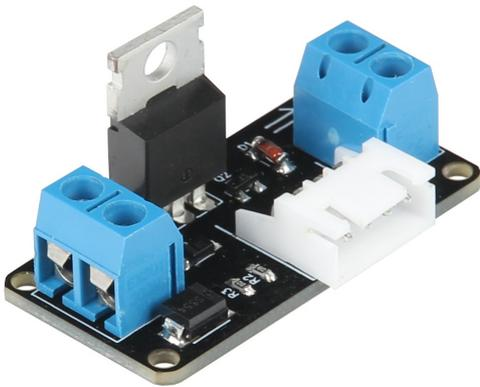
With this MOSFET, you can control a voltage of up to 36 Volts. With the pulse width modulation, the root-mean-square voltage can be lowered (f.e. to dim a LED light).
