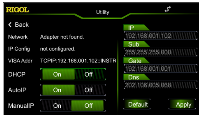
Figure 2-26 LAN Setting Interface
