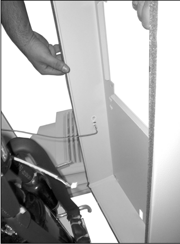
Fig. 72: Disconnect the earthing cable (1)
