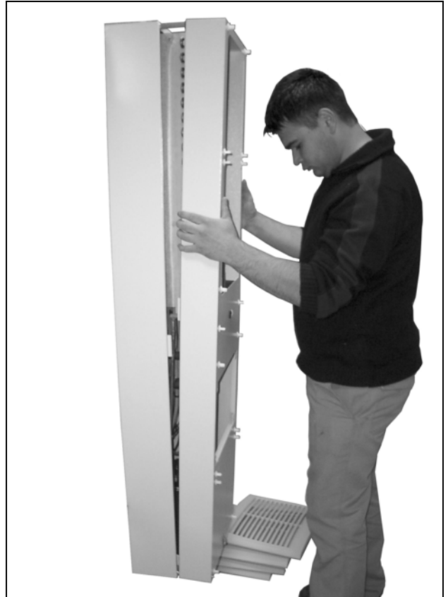
Fig. 71: Removing the cover
