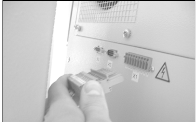
Fig. 53: Disconnect the mains plug
