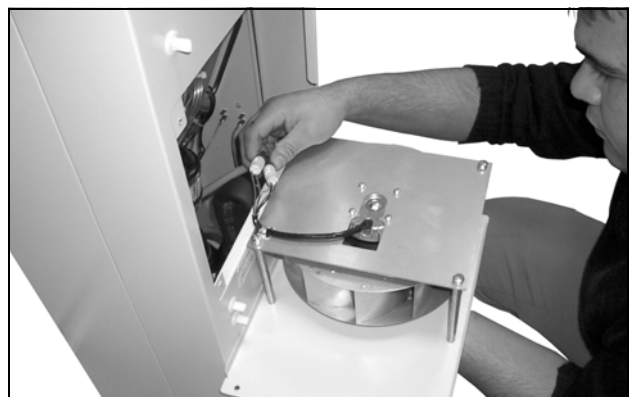
Fig. 65: Disconnect the fan connectors (1)
