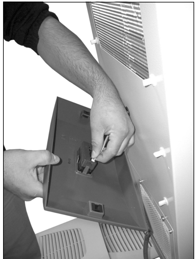
Fig. 38: Disconnect the connector from the display (1)
