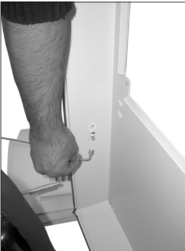
Fig. 73: Disconnect the earthing cable (2)
