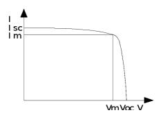
The solar cell can generate a wide range of voltages (V) and currents (I). As the resistance of the connected electrical load increases continuously, from zero (a short circuit) to an extremely high value (an open circuit), the maximum power output can be determined.
