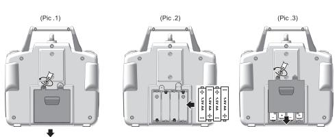
ATTENTION: Batteries shall be put to the right polarity.
