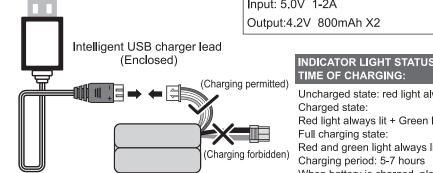
7.4V 2000mAh Li-Ion (Enclosed)
