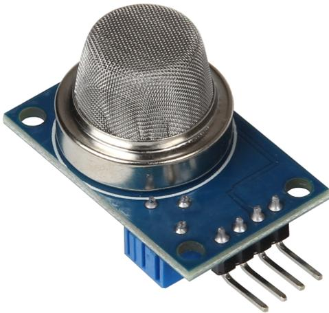
This analog gas sensor has a small heating part with an electronical chemical sensor. It is suitable for indoor usage. The sensor can output exact values only after warm-up phase.
