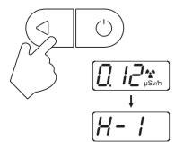
To enter the settings mode, it is necessary to press and hold the mode button in the radiation background measurement mode
