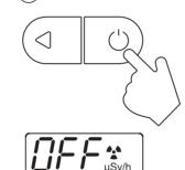
To turn off the device, it is necessary to press and hold the power button until the inscription appears on the display « UFF »
