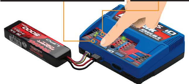
Press and hold the Start button(s) for 1 second. The charger will play a tone, indicating that charging has started. Press once to stop. The charger will play a tone, indicating that charging has been canceled. The charge progress LEDs will light as the battery charges.
