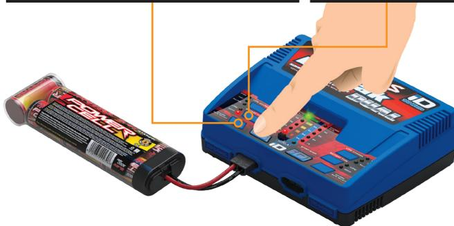
Press and hold the Start button(s) for 1 second. The charger will play a tone, indicating that charging has started. Press once to stop. The charger will play a tone, indicating that charging has been canceled. The charge progress LEDs will light as the battery charges.
