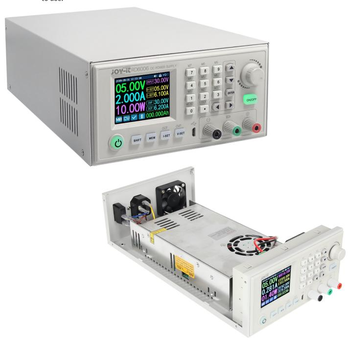
You can adjust with the help of the fine-tuning potentiometer the output voltage of the RD6006-NT. You can see your adjustment at the input voltage of your RD6006. Ideally, the RD6006 has a input voltage of 65 V to be able to issue the complete 60 V.
