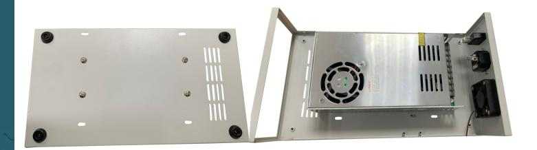
5. Srew now the fan controll in the case next to the power supply with the remaining black screws and connect the fan with the according connection.
