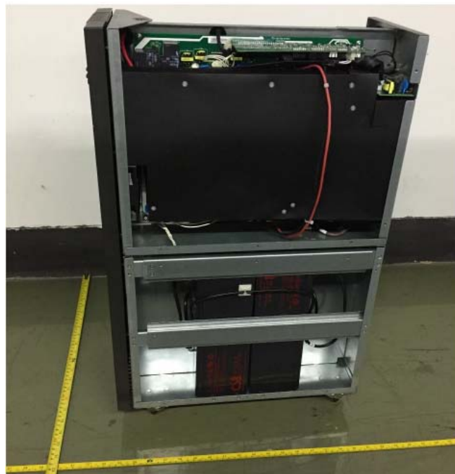
Figure 6 M/N: SRVb10KI General Internal of the E.U.T.
