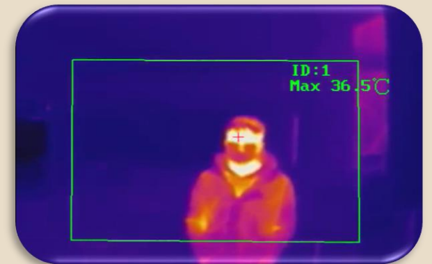
Fast fever screening with abnormal temperature alarm (pop-up image/audio warning)
