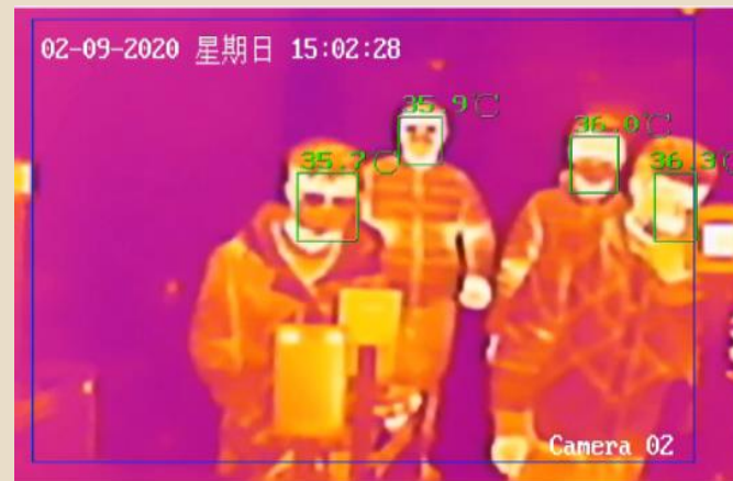
Skin-temperature based detection in high accuracy ( \pm 0.5^{\circ}\text{C} ) without surrounding interference; simultaneous fever screening for up to 30 persons
