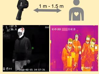
Skin-temperature based detection in high accuracy (±0.5°C) without surrounding interference Fast fever screening with elevated temperature alarm (pop-up image/audio warning)
