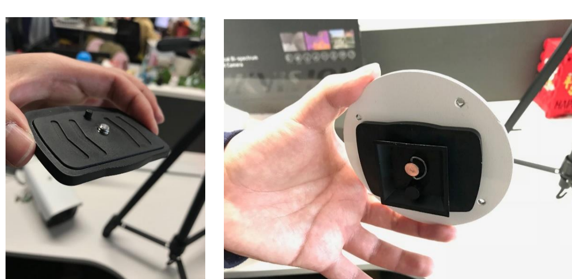
A. Tripod connector fixed on the adapter
