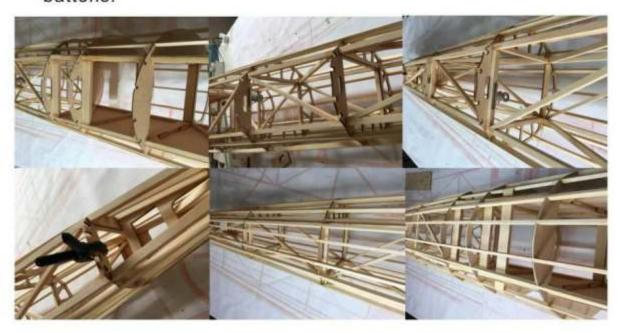
15) Assemble and glue the servo mount on fuselage.
