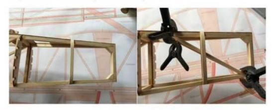
Stick the fuselage battens, some ones need to be butted joint and extended.
