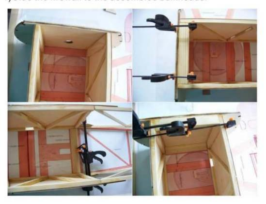
5)Stick the wooden strip according to the red position(3D drawing)
