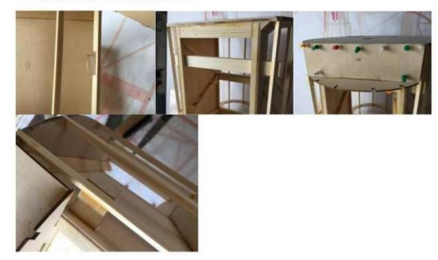
13) The 6X8MM batten was cut out, and the 10X28X270MM batten was inserted to stick and fix, and the redundant part was cut out.
