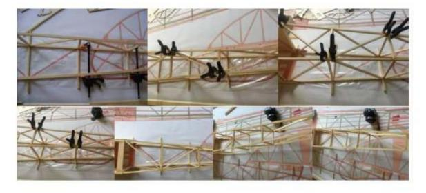
7) Assemble and glue the fuselage bulkhead.
