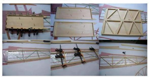
3)Assemble the bulkheads(front&back).
