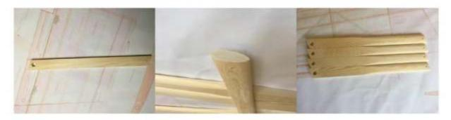
18) Align the finished struts with the drawing and mark the mounting position.
