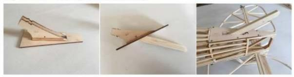
33) Fill with wood chips to make holes for servo arm.
