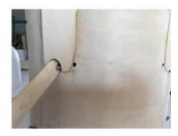
30) Assemble landing gear assembly and install steel wire stay.
