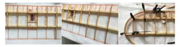
5) Stick and polish the lower wing face reinforced wood blocks.
