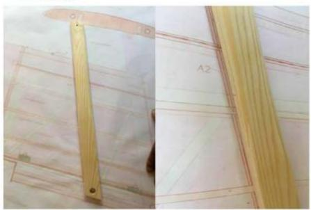
Cut off the bar which block the strut, and align the strut with the fuselage and fix it.
