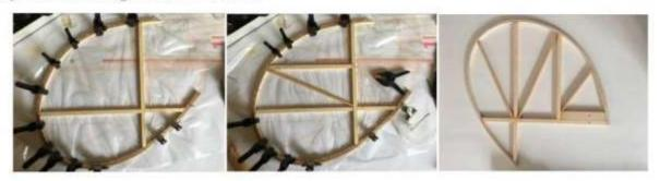
8)Provisionally fix the horizontal tail, adjust the distance between the two sides to be equal.
