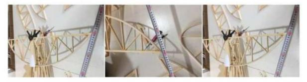
9)Mark from the bottom screw holes, drill the 3MM holes, and use the 3MM screw rods to fix from the bottom.
