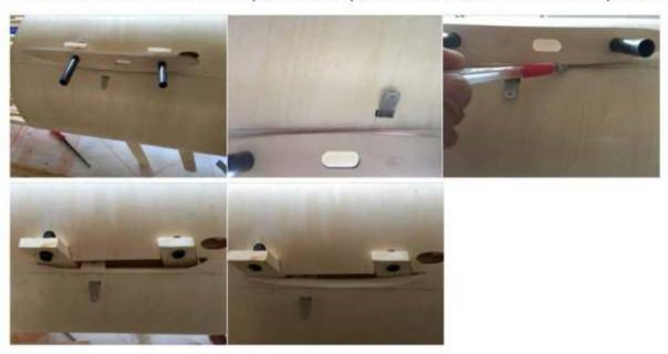
27) Dig a threading hole in the marked position.
