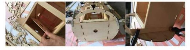
9) Cut off the excess wood and paste the A19 plywood.
