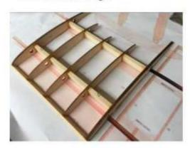
4)Attach the wing ribs to the trailing edge.
