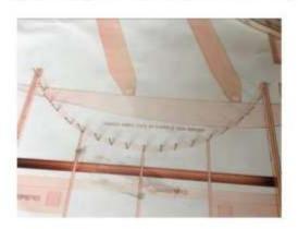
Dip the balsa in water to make it easier to bend. Then paste after drying.
