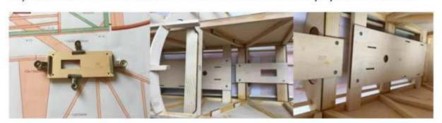
17) Struts: Drill holes of 3MM and 12MM on the struts according to the position in the drawing, and polish the wood into an oval shape.
