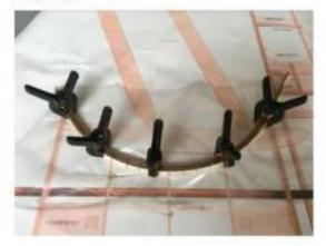
Paste the wing ribs according to the drawing.
