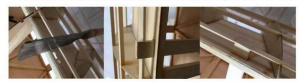
14) Install the bottom bulkheads of the fuselage and stick the fuselage battens.
