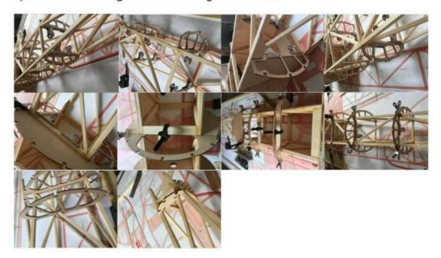
8) Glue the firewall stiffener plate and triangular stick.
