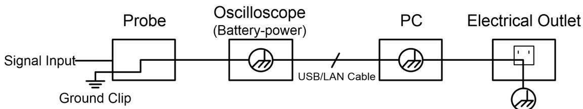
It is not allowed to measure AC power when the oscilloscope is AC powered, or when the battery-powered oscilloscope is connected to the AC-powered PC through the ports.
