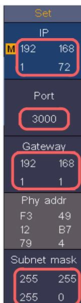
Figure 5-7 Set the network parameters of the oscilloscope
