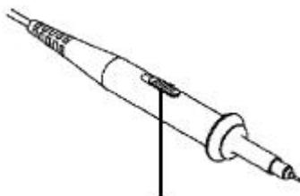
Figure 3-8 Attenuation Switch
