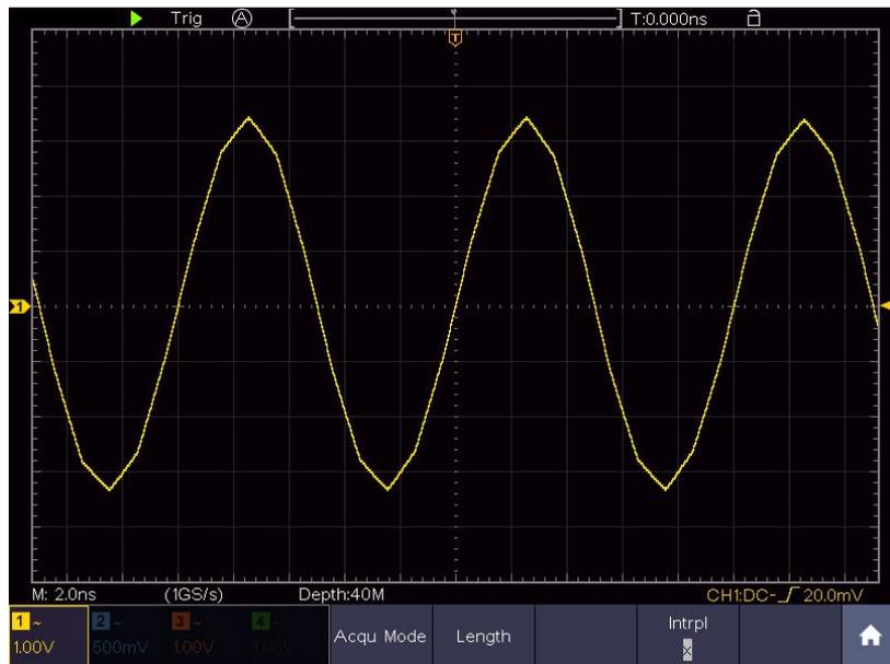
Figure 4- 5 Linear interpolation
