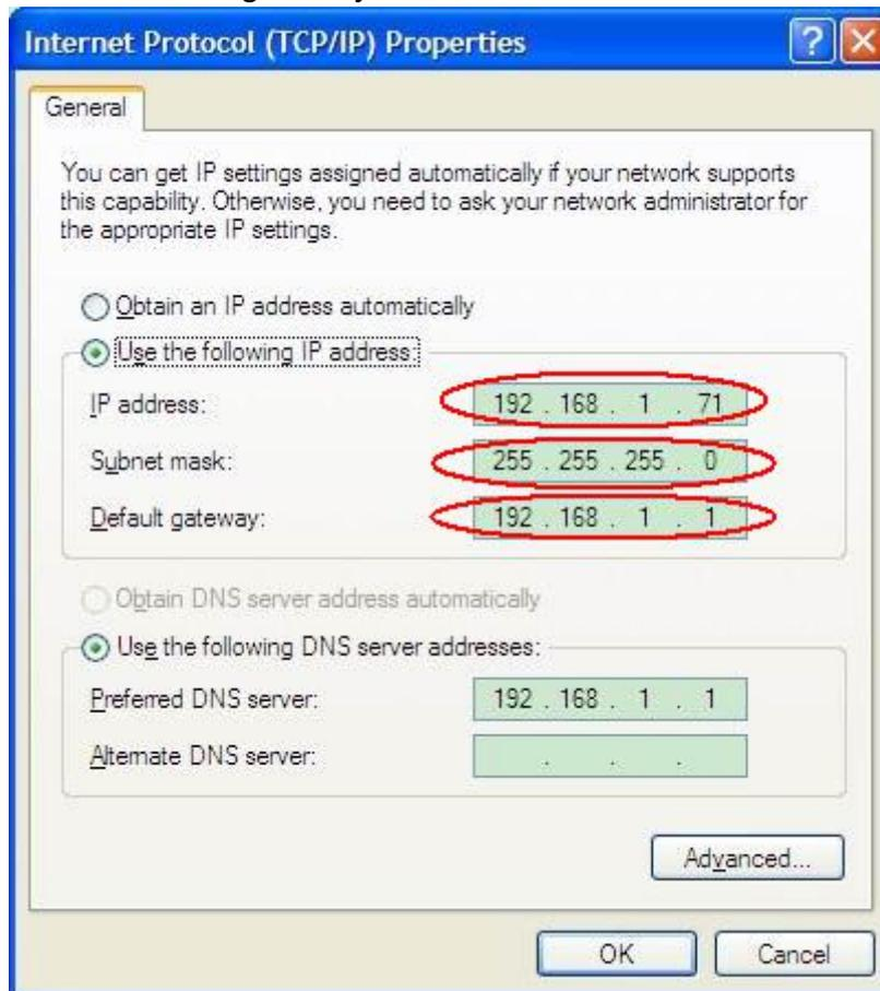
Figure 5- 5 Set the network parameters of the computer
