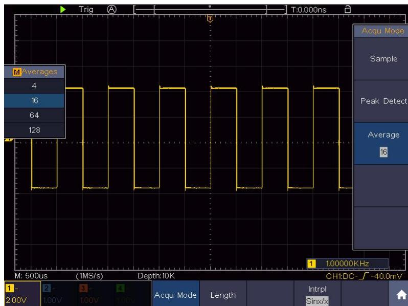
Figure 6-5 Reduce Noise level by using Average function
