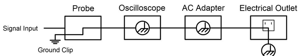
The diagram of the ground wire connection when the battery-powered oscilloscope is connected to the AC-powered PC through the ports:
