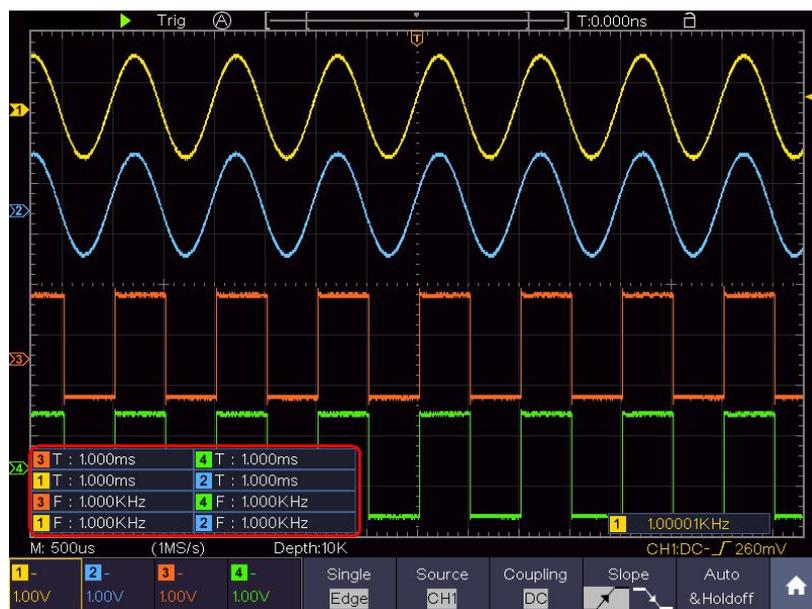
Figure 4- 18 Automatic measurement
