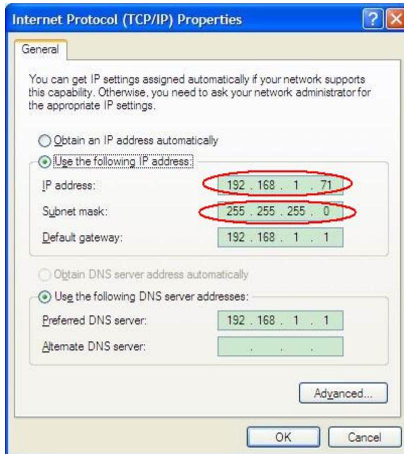
Figure 5- 2 Set the network parameters of the computer
