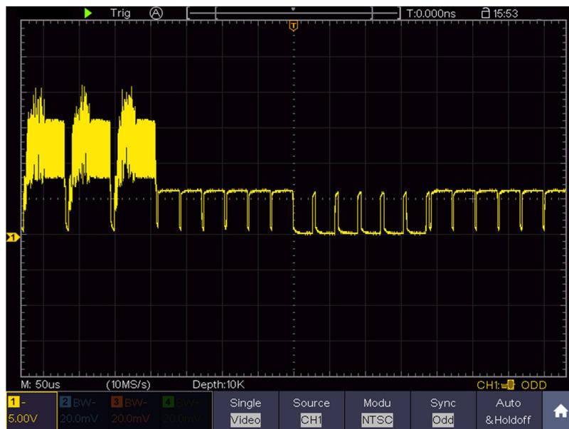
Figure 6-7 Waveform Captured from Video Field Trigger
