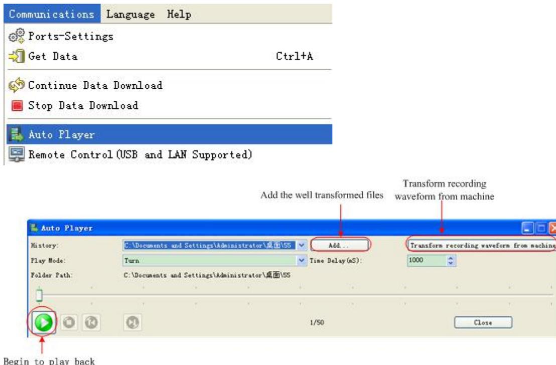
Figure 4- 17: Play back waveform by software
