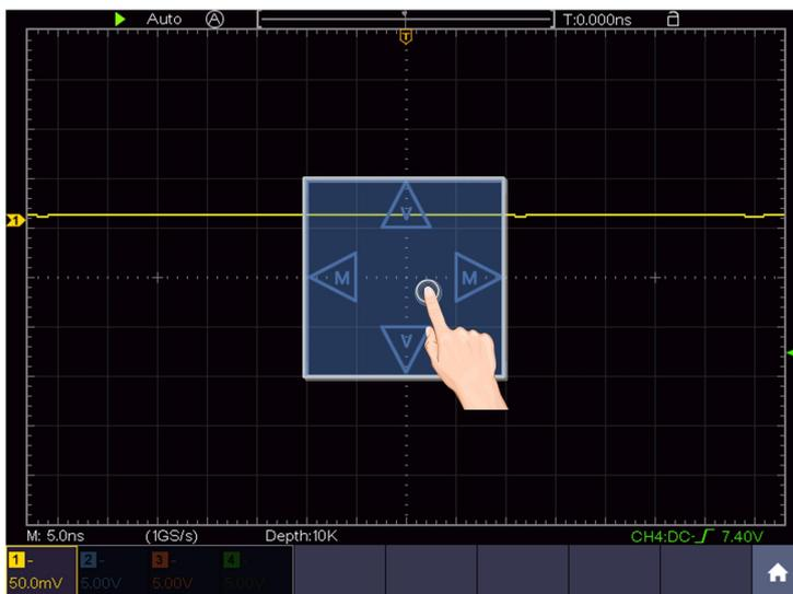
When the **M** and **V** icons appear, in the full screen, swipe left/right to change the time base, swipe up/down to change the voltage division of the selected channel.
