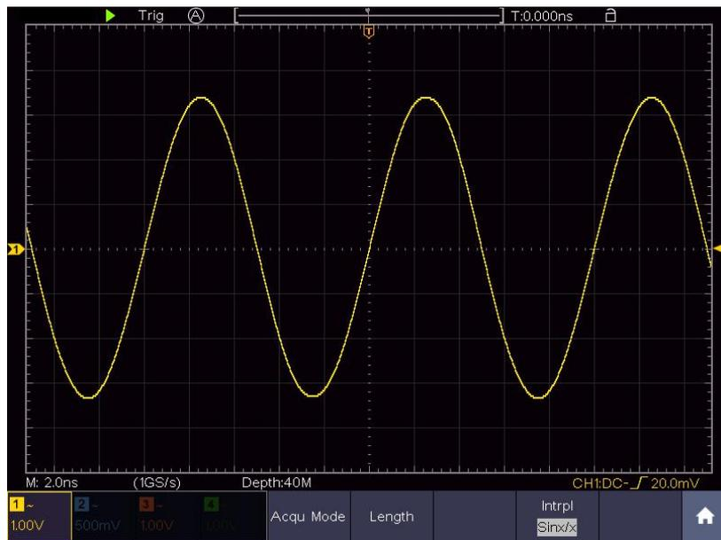
Figure 4- 4 Sine(x)/x interpolation
