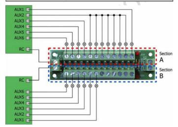
If more than 12 connections are required, the two sections can be connected by connecting the two connectors of X2. Then, however, only one circuit may be connected!
