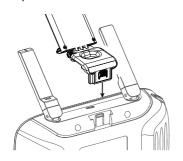
Install the mobile phone support in the slot of the back of the remote controller.
