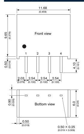
$\begin{array}{l} \mbox{Dimensions in mm (inch)} \\ \mbox{Tolerances: } x.x \pm 0.5 \ (x.xx \pm 0.02) \\ x.xx \pm 0.25 \ (x.xxx \pm 0.01) \\ \mbox{Pin dimension tolerance: } \pm 0.1 \ (\pm 0.004) \end{array}$
