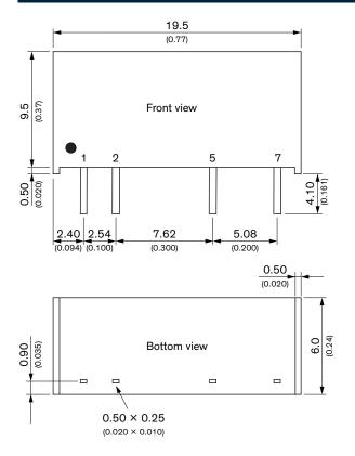
$\begin{array}{l} \mbox{Dimensions in mm (inch)} \\ \mbox{Tolerances: } x.x \pm 0.5 \ (x.xx \pm 0.02) \\ x.xx \pm 0.25 \ (x.xxx \pm 0.01) \\ \mbox{Pin dimension tolerance: } \pm 0.1 \ (\pm 0.004) \end{array}$
